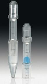
Vivaspin® ultrafiltration concentrators are disposable devices for biological samples. Vivaspin<sup>®</sup> 500 is suitable for sample volumes from 100-500 µl while Vivaspin<sup>®</sup> 2 can handle samples up to 2 ml. The patented vertical membrane design and thin channel filtration chamber (US 5,647,990) minimizes membrane fouling and provides high speed concentrations.
