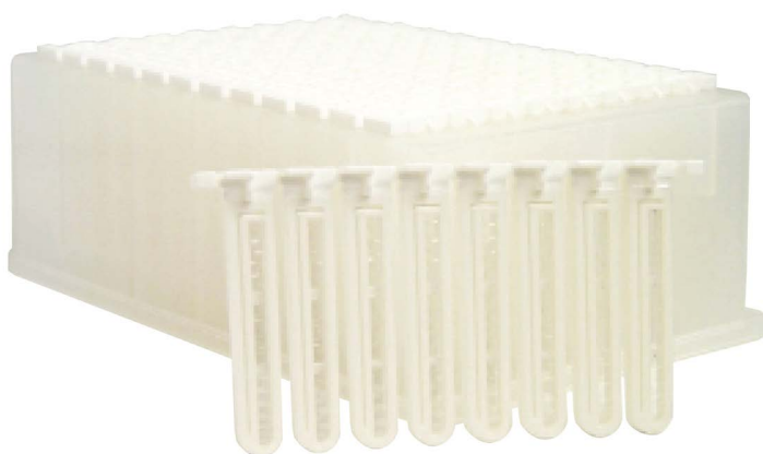
Figure 5 | 96 deep well plate Riplate (Ritter Medical) with 12 cartridges ED300 (scienova GmbH) dialysis cartridges for 96-fold dialysis
