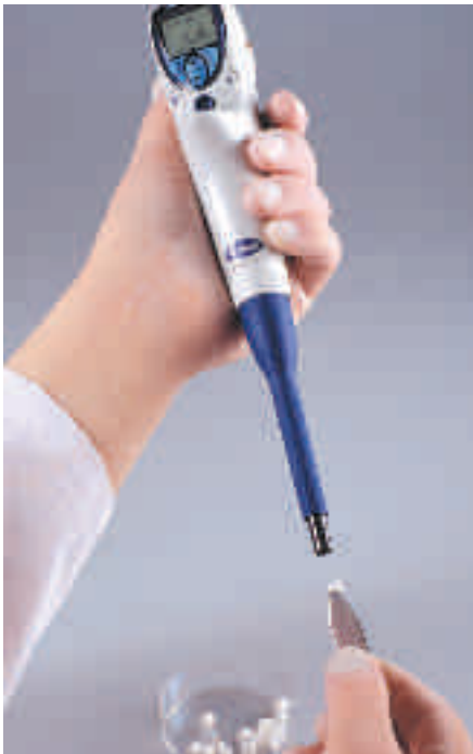
Fig. 2: The filtered tip cones protect pipettors from contamination and samples from carry-over. Forceps packed with each pipettor enable the easy and clean placement and removal of the filter.
