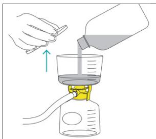
3. Immediately after mixing the filter aid with the cell culture broth, remove the dust cover from the funnel, pour the cell culture | filter aid mixture into the Sartolab® RF | BT and place the dust cover back on. Then apply vacuum to the filtration unit to filter.
