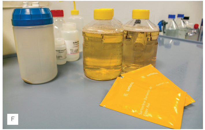
Figure 2: Pouring in and clarification of mammalian cell culture supernatant with 40 g of filter aid using the filter unit Sartolab® RF included in the Sartoclear Dynamics® Lab kit (A – F). A tube is connected to a vacuum pump.
