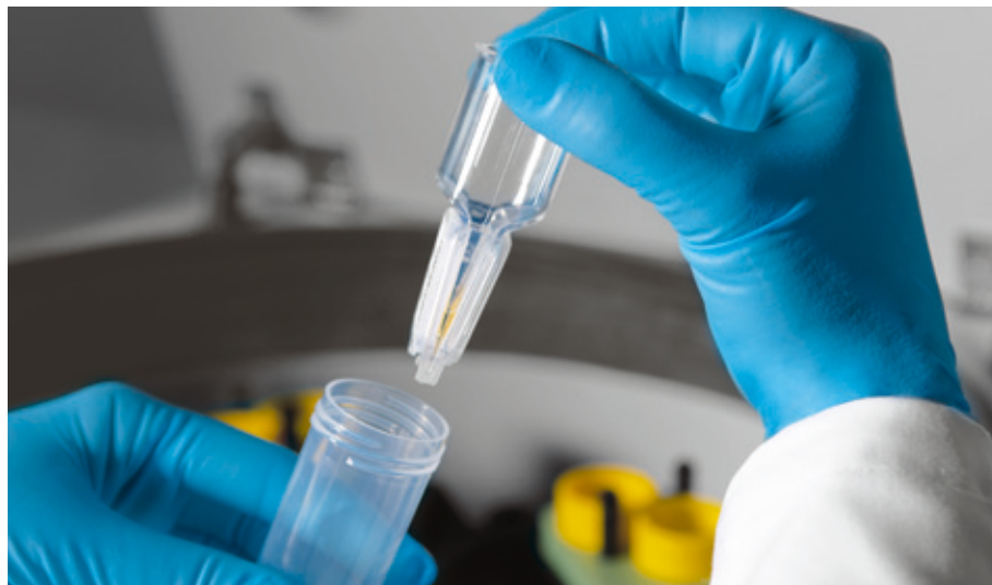
Disposable Ultrafiltration device for sample concentration
