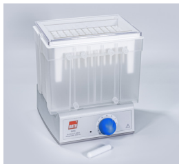
Figure 10 | XDB Dialysis Box with peristaltic pump
